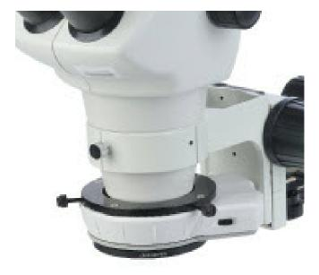
SHOWN WITH POLARIZER / ANALYZER KIT INSTALLED
